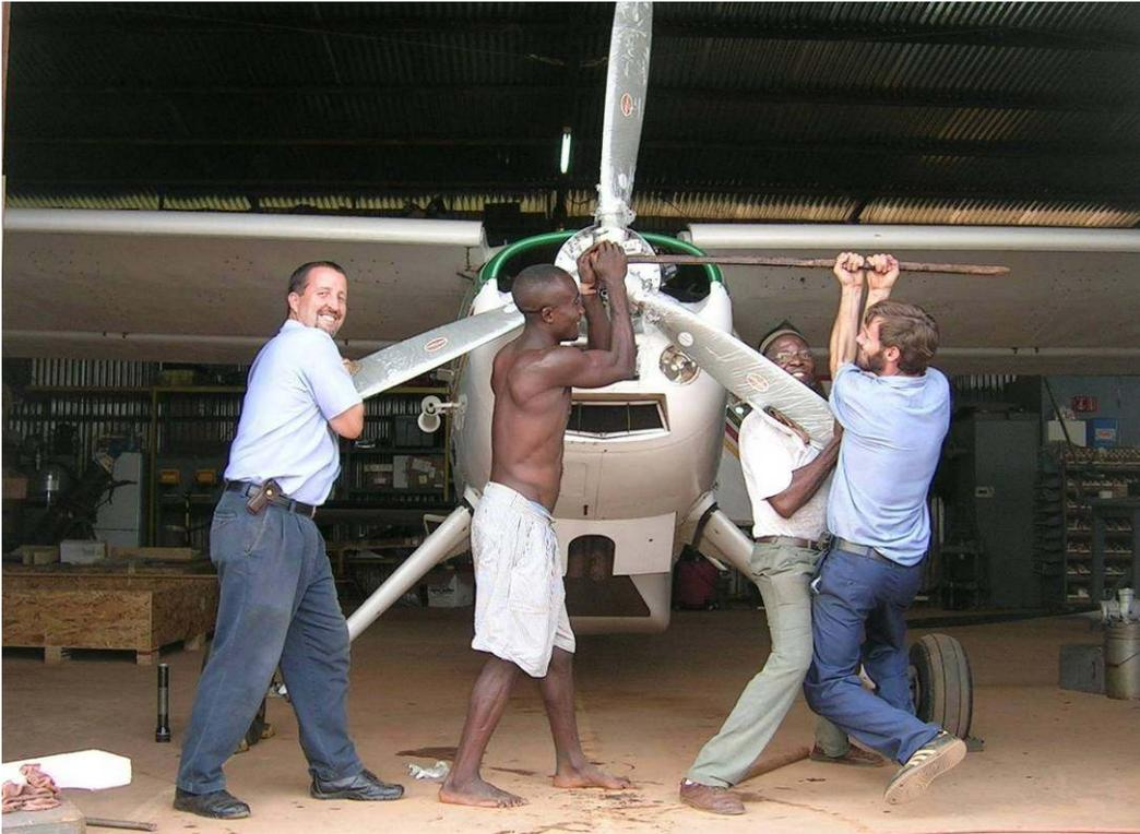
*Torquing the propeller to 450 ft. #*
