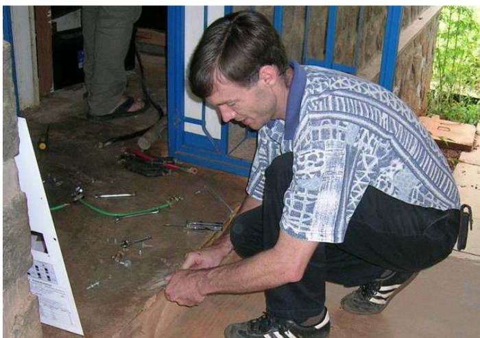
*Filing battery connectors for the Smith's solar system*
