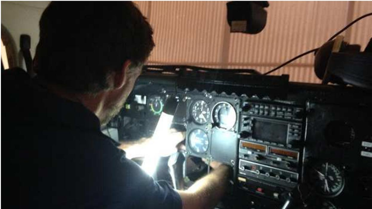
*Working to re-pin the instrument connectors. See also Steve Straw's [blog](#) for additional detail.*
